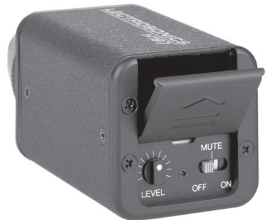
On the H187 transmitter, the LEVEL control on the rear panel and LEVEL and LIMIT LEDs on the top panel next to the input connector are used to set the input gain for optimum signal to noise ratio.
