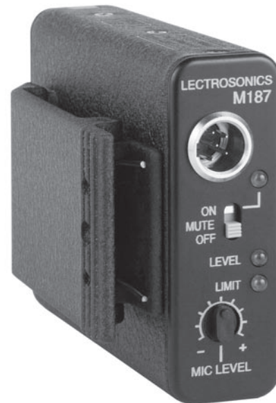
On the M187 transmitter, the MIC LEVEL control and LEVEL and LIMIT LEDs are used to set the input gain for optimum signal to noise ratio.
